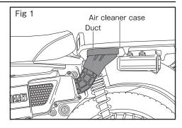
2) Remove the center cover, side cover, and air cleaner cover in this order. (Fig 2)
